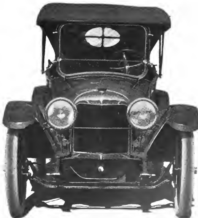
Front view of 1915 Oakland, showing streamlines of the hood and body and V radiator
